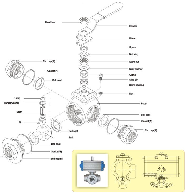
ISO direct mount for actuator assembling directly.
